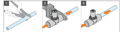
To make the connections quickly and correctly, it is essential to use tools that comply with the DVS2207 standards. The welding procedure must comply with the DVS2207-2208 joint standards.
