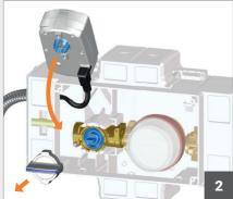
Remove the handle and insert the €100 electric actuator into the valve seat with light pressure.
